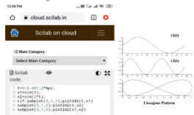
FIG. 11: SciLAB plotting on cloud, for Lissajous pattern when \theta = 0^\circ and v_1 = \sin(t) ; v_2 = \sin(2t)
