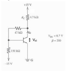
+15V = (I<sub>C</sub>+I<sub>B</sub>)R<sub>C</sub>+ I<sub>B</sub>47k Ω + I<sub>B</sub>150 kΩ-15V
