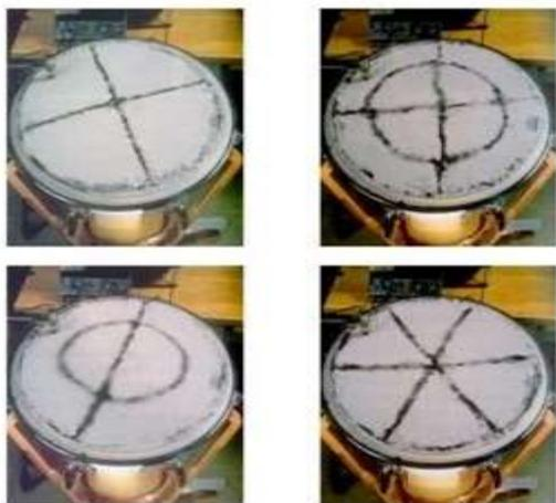
**Figure 2: Standing waves in drum**
