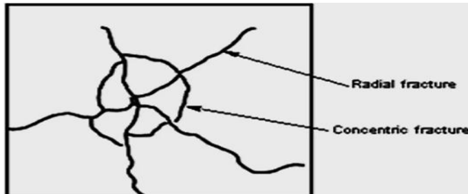
Glass Fractures hit by a bullet
