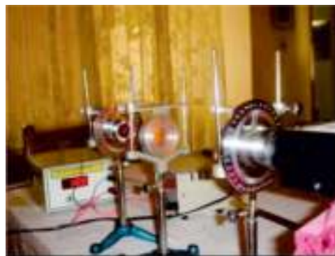
Fig 4: A QWP is inserted between the crossed polarizer and the analyzer
